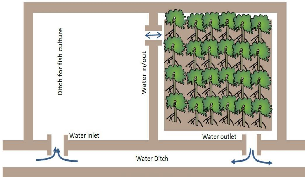
Model 6 (Type 2): Open fishpond type (Model Empang Terbuka) with two-gate water inlet system, elevated bank (Sofiawan, 2000). Officially recognised by the Ministry of Forestry (2004) as the fourth of four silvo-fishery options. Local communities tend to use this option, some also without the elevation. It is then known as the tanggul model. Illustrations by Audrie Siahainenia.
