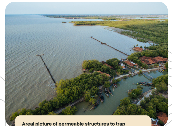
Areal picture of permeable structures to trap sediment to enable mangrove regrowth along the eroded coastline of North Java © Boskalis
