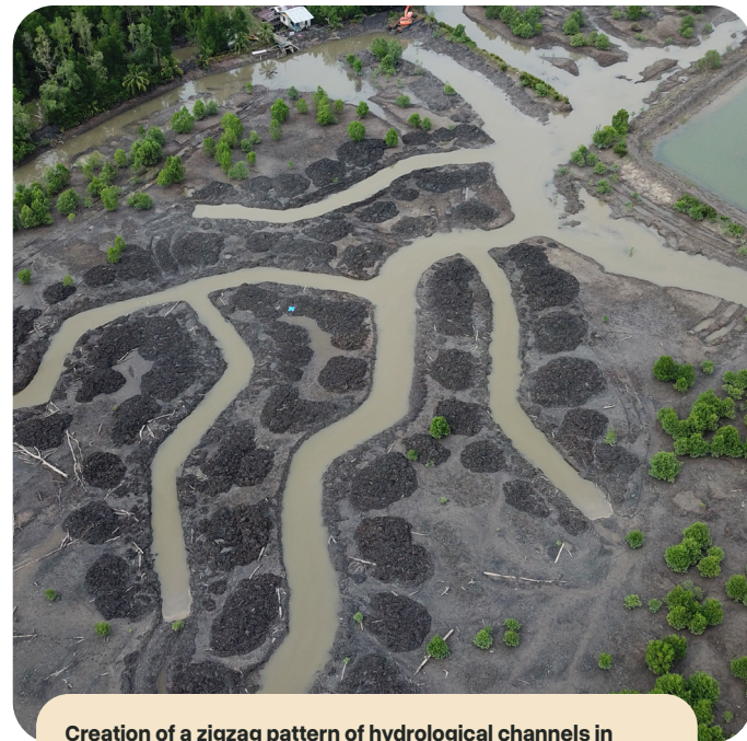
Creation of a zigzag pattern of hydrological channels in North Kalimantan to mimic the natural flow pattern and enable mangrove propagules and seeds from nearby healthy mangroves to reach the abandoned ponds © Wetlands International
