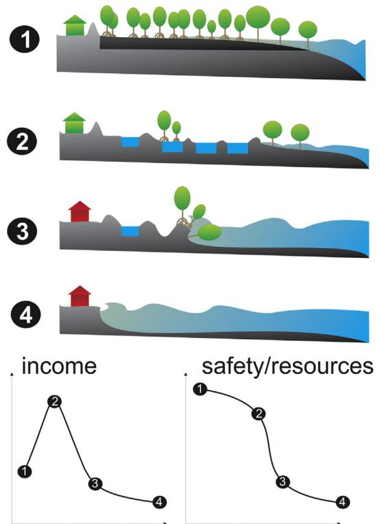
**Fig. 2.** Development of income, flood safety and resources for communities along mud-mangrove coasts. 1. Natural mangrove forest with small fishing or agricultural communities, 2. Large-scale mangrove cutting and intensive aquaculture, 3. Reduction of pond yield and start of coastal erosion, 4. Large-scale coastal erosion and increasing salinity intrusion.
